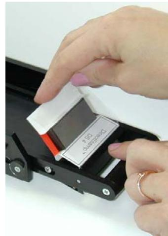
9. Keep the folded edge fully inserted in the slot and push the drawer into machine.
